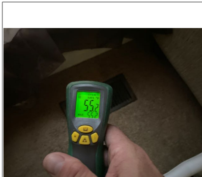
Air conditioning temperature at register for 4928
