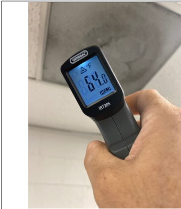
Several of the air conditioning systems were not cooling properly. Recommend repair by qualified HVAC technician.
