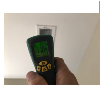
Heating system two temperature at register
